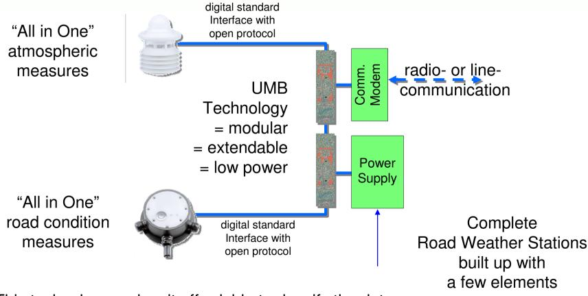
This technology makes it affordable to densify the data acquisition network in order to enhance the capability of providing optimal Road Weather Condition Information
