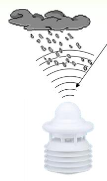
24 GHz microwave doppler radar measures velocity and dimension of nucleus in order to detect type and intensity of precipitation
