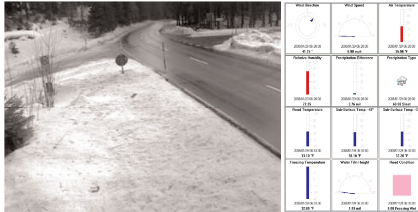
figure 7 Example picture and indicator display of data from a road site in Bavaria
